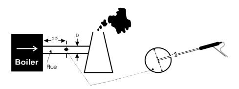
Use the probe's depth stop cone to fix it in flue diameters from  $^{1}/_{4}$  to  $^{4}/_{5}$  inch, 6 to 21 mm. Its maximum operating temperature is  $1112^{\circ}F / 600^{\circ}C$ .
