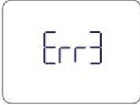
The monitor is measuring temperature outside its measurement range.
