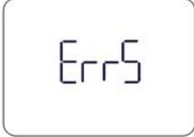
These are displayed when it is necessary to reset the monitor. To reset, switch off the monitor, remove its batteries and wait for a minimum of one minute, reinsert batteries and switch on. If either error message remains please contact our Service Department for further assistance.
