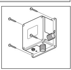
Make sure that the rubber washers are in place in the flexible pipes. Connect the flexible pipe from the tap to the bottom outlet marked 'Water Out'. Connect the other flexible pipe to the side connection marked 'Water In'.
