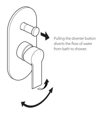
Moving the control lever anti-clockwise will decrease the water temperature.
