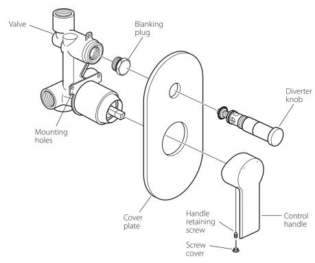
Before installing your new mixer, flush through the pipe work to ensure removal of debris, turn off the water supply.
