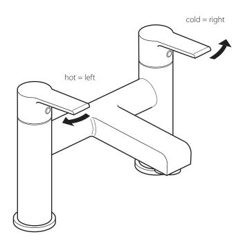
Moving the levers in the direction of the arrows will increase the flow of water.
