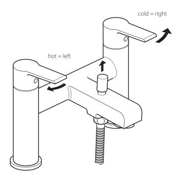
Moving the levers in the direction of the arrows will increase the flow of water. Pull the diverter knob up to turn on the shower.
