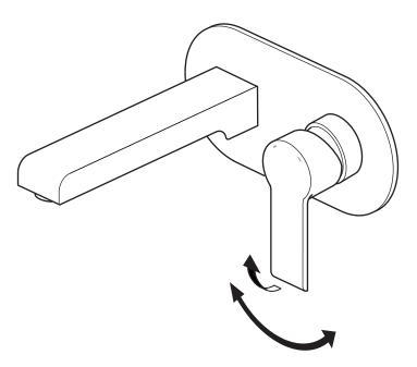
Moving the control lever anti-clockwise will decrease the water temperature.
