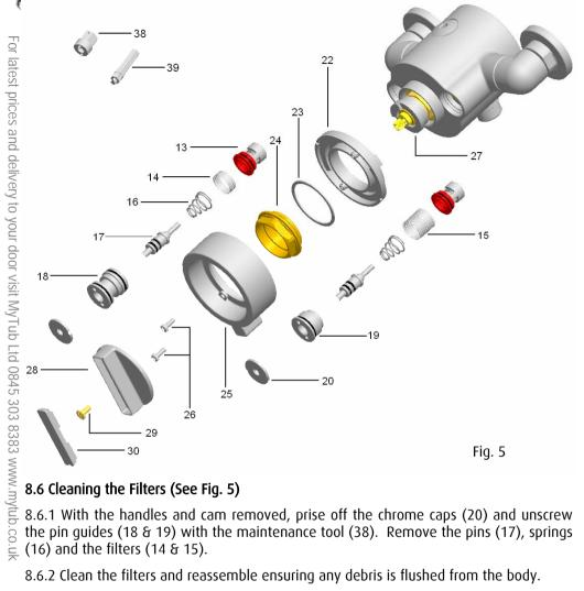
8.6.2 Clean the filters and reassemble ensuring any debris is flushed from the body.
