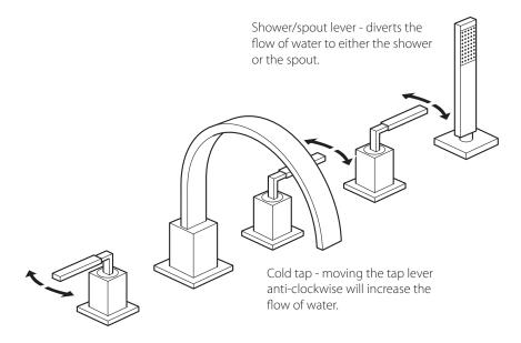
Hot tap - moving the tap lever anti-clockwise will increase the flow of water.
