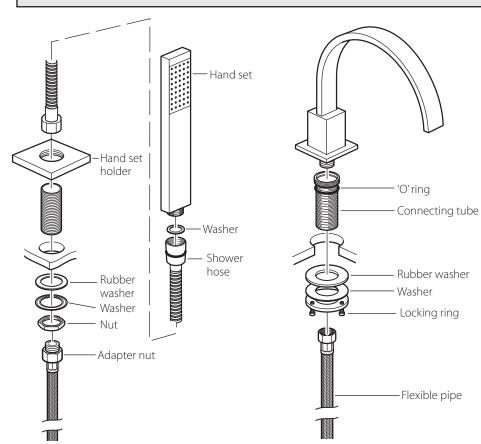
Position Hand set holder in the hole, from the underside slide on the rubber washer, and then the nut.
