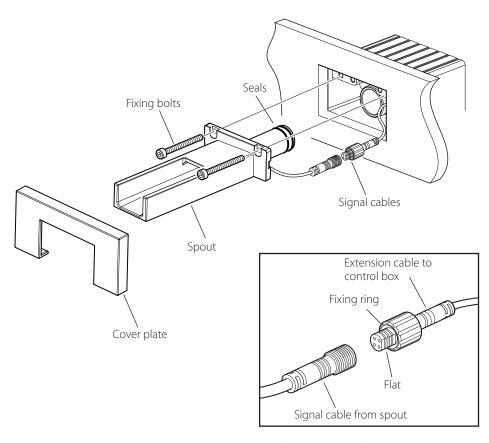
Flush through the pipe work to ensure removal of debris, turn off the water supply. Prepare the short extension coming from the control box to the spout, push through the hole in the side of the installation box making sure that the correct end is coming out of the wall (with the fixing ring).
