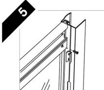
Screw together using the 15mm dome head self tapping screws provided.
