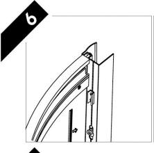
Fit seal between glass and aluminium
