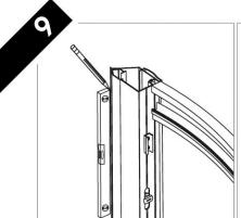
Check the wall profiles are vertical and mark their positions on the wall. Then remove the frame from the tray.
