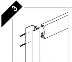
In the same way, fit the top curved rail to the inner wall profiles, left and right. Left profile shown.
