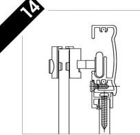
With the frame secured to the wall we can now hang the doors into the outer track slot.
