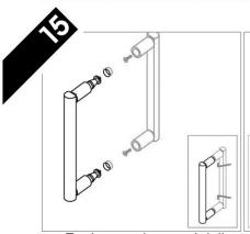
Now fit the handles, as shown, with the grub screw section on the outside of the enclosure.
