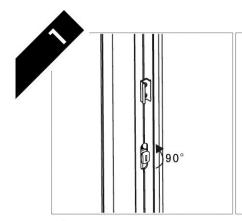
Part the inner and outer wall profiles by rotating the key inline with the slot.
