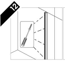
Screw the wall profiles to the wall using the 30mm screws provided.
