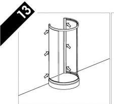
Place the assembled frame and glass back onto the tray and secure to your fixed wall profiles using the micro adjusters.
