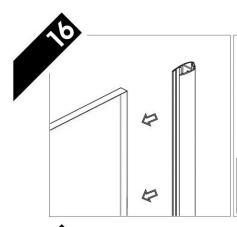
Fit the magnet seal to the leading edge of the doors.
