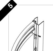
Screw together using the 15mm dome head self tapping screws provided.
