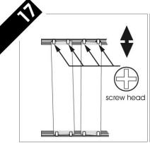
If the doors are misaligned, use the adjusters on each top roller to ensure the seals fit together easily.
