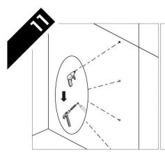
Drill the holes where marked using a 6mm drill bit (you may need a specialised drill bit if you are drilling into tiles, if unsure please seek advice).
