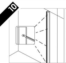
Remove the outer wall profiles from the frame (key slot) and position onto the wall in your marked position. Then mark through the fixing holes in the profile. Repeat for both sides.
