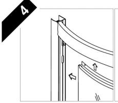
Fit the glass panels into position, aligning the holes to those in the top rails.
