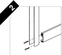
Fit the bottom curved rail to the inner wall profiles, left and right. Left profile shown.
