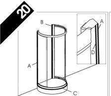
Using good quality silicon sealant, seal the enclosure to the wall and tray along the following joints:
