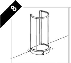
Place the assembled frame and glass onto the tray and adjust the micro adjusters so that the frame sits slightly in-board from the edge of the tray.
