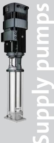
MTA > The lower performance range up to 100 l/min and delivery heights up to 10 m are attended to by immersible pumps of the MTA series. Their robust construction with open stainless steel impeller makes them suitable for media with increased viscosity and corrosiveness, as well as for high solids content. This is why the MTA series is preferred for cooling lubricant supply during lathing and parts cleaning.
