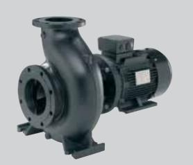
**MTPO** > Single stage, self-priming recirculation pump in closed-coupled design, with mechanical seal. Its special construction makes the MTPO suitable for delivery of highly aerated emulsions and oils. Maximum delivery is 350 l/min.
