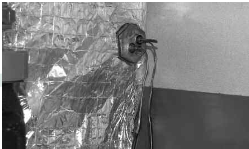
Figure 10-3: Thermostat phial position
