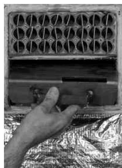
Figure 11-1: Removing the baffles
