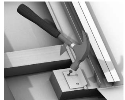
Figure 63: Securing Side Gutter Clips
