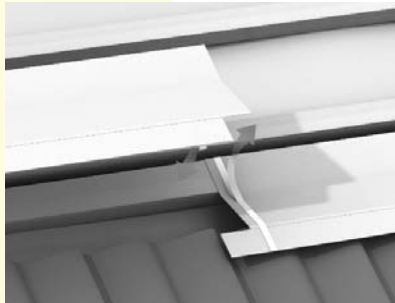
Figure 55: Installation of Additional Bottom Flashings
