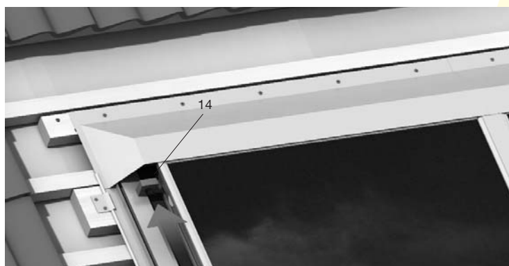
Figure 74: Fitting Foam Block (14)
