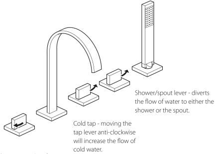
Hot tap - moving the tap lever clockwise will increase the flow of hot water.
