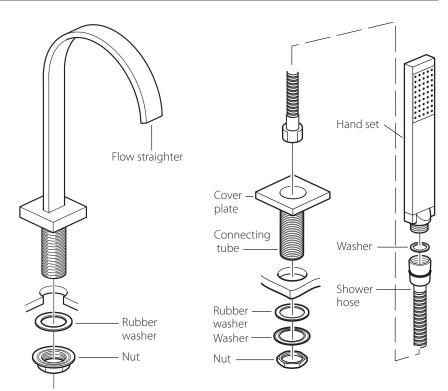
Ensure that the 'O' ring is in place in the underside of the cover plate.
