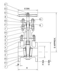
Crane cast iron gate valves offer the ultimate in dependable service wherever minimum pressure drop is important. Each valve is hydrostatically tested to BS5150
