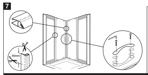
Trim the seals (PN40042) to the length of the glass. Cut 40mm off the seal flap at the top and bottom and push-fit onto the back edge of each door with the flap as shown.
