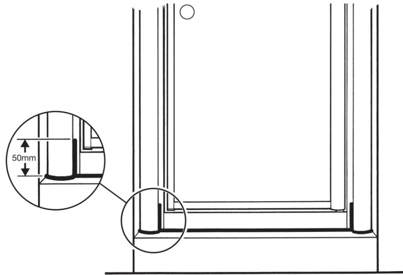
**GB** From the outside only, apply sealant to the bottom of the enclosure and 50mm up the wall channels as shown.
