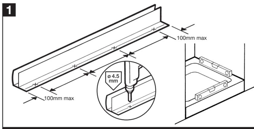
**GB** Drill holes in both wall channels at points shown using a 4.5mm drill bit, through the edge shown and in the grooves. Ensure shower tray is level in all directions.
