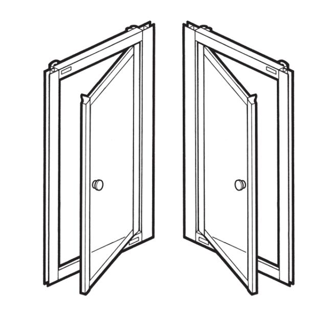
**GB** Fit the door handle to the door ensuring the supplied handle washers are used on each side of the glass. A chrome finish handle is supplied with all frame finish options. Choose the opening side for the door (turn over if necessary).
