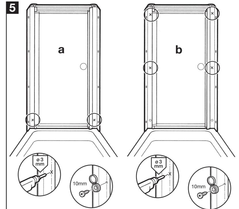
**GB** Check door is centrally positioned and perfectly vertical. Drill inside of wall channels using 3mm drill bit in the two lower positions shown. Fix using 10mm screws and screw caps (a). Check door is vertical, drill next 4 holes and fix using 10mm screws and screw caps (b).
