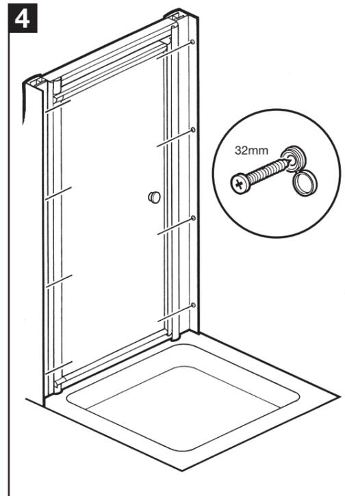
**GB** Place door in position on the tray, fix wall channels to walls using 32mm screws and screw caps.
