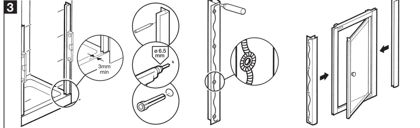
**GB** Place wall channels on tray ensuring they are vertical and a minimum of 3mm back from the front of the tray. Place masking tape against the wall before marking drill hole positions. This will help prevent the drill bit slipping. Drill 6.5mm holes, 30mm deep and insert wall plugs. Apply sealant to the back of wall channels. Place wall channels onto door.
