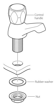
Before installing your new tap, flush through the pipework to ensure removal of debris, turn off the water supply.
