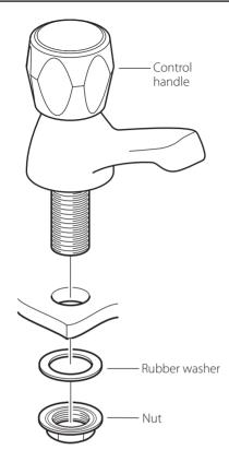
Before installing your new tap, flush through the pipework to ensure removal of debris, turn off the water supply.
