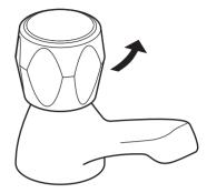
Turning the cold handle anti-clockwise will increase the flow of cold water.
