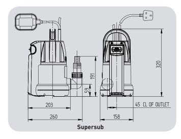
All models are supplied complete with a G  $1^{1\!/_2}$  M x G  $1^{1\!/_2}$  M x 90° elbow and a G  $1^{1\!/_2}$  F stepped hose connector, suitable for 25, 32 or 38 mm bore hose.
