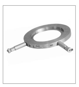
Danfoss flow measuring orifices are used to precisely determine the flow in water based heating, cooling or potable water systems. This determination is done by measuring the differential pressure across the fixed orifice, which has a well known Kv value.
