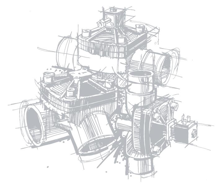
2-way solenoid valves with Clip-on coils for neutral liquids and gases
