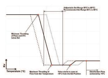
\* The performance chart above indicates the shift in thermal reaction when the temperature set point of 57°C is altered.
